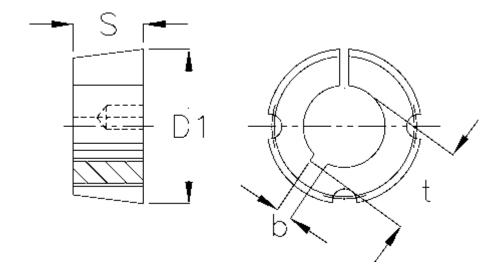
$\begin{array}{lll} b & = 14 \\ Bore & = 45 \\ Bush type & = 3020 \\ D1 & = 108 \\ S & = 50,8 \\ Screw size & = 5/8 \times 1 \ 1/4" \\ t & = 48.8 \end{array}$
